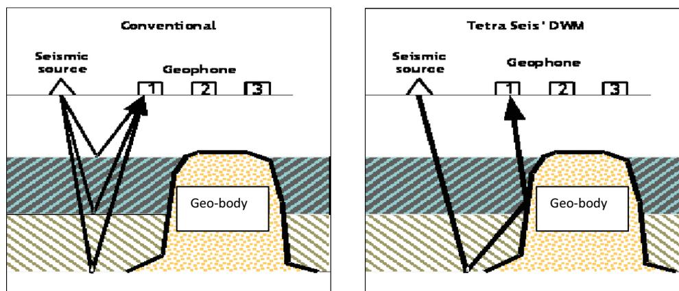
Figure 2, Direction of wave propagation which is used in conventional and Duplex Wave Migration Method.
