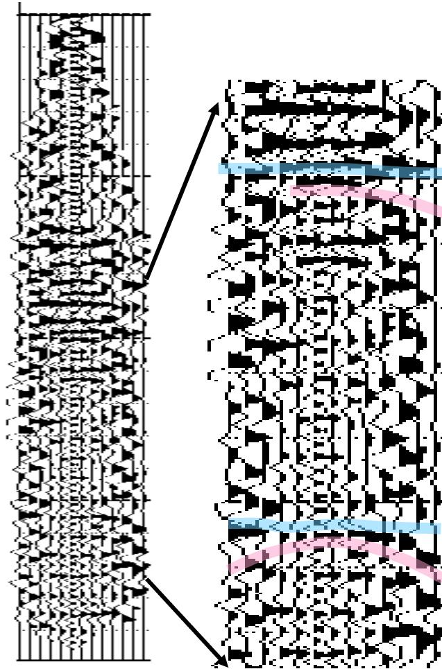
**Examples of synthetic CDP gathers** used in calculation of parameters of multiples.
