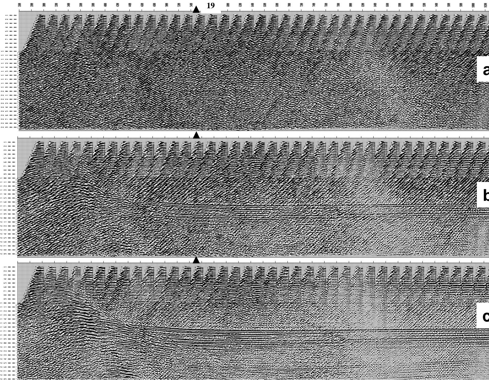
**Comparison of synthetic time cross-sections obtained for the flank scheme with step between centers of groups  $\Delta X_{RP}=40$  m:** a – without receivers grouping; b – grouping of receivers on base  $I_G=80$  m; c - grouping of receivers on base  $I_G=120$  m.
