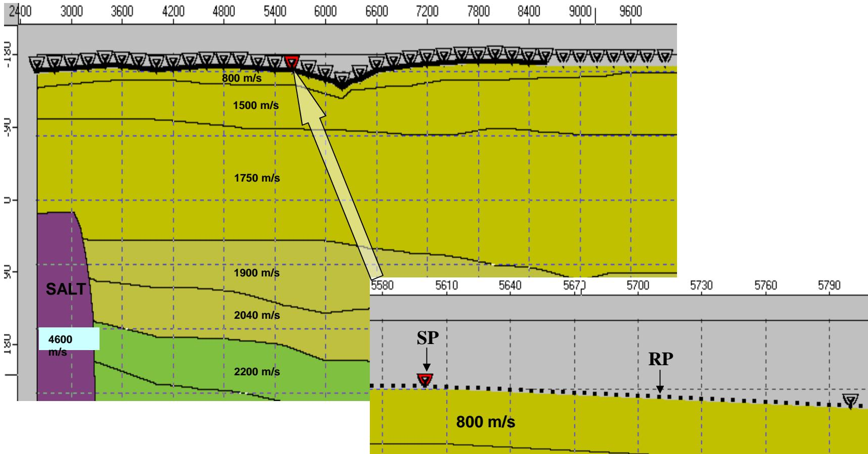
Detailed model of low velocity zone (LVZ) for this survey site
