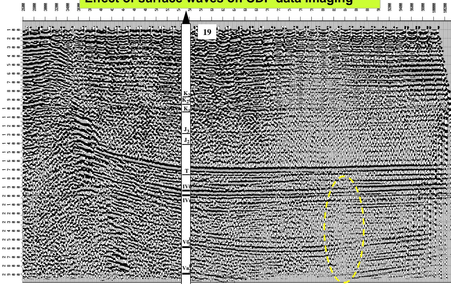
Synthetic time cross-section obtained for **the central scheme** with receiver grouping on base  $I_G=150$  m and interval between centers of a group  $\Delta X_{RP}=50$  m (magnified scale).
