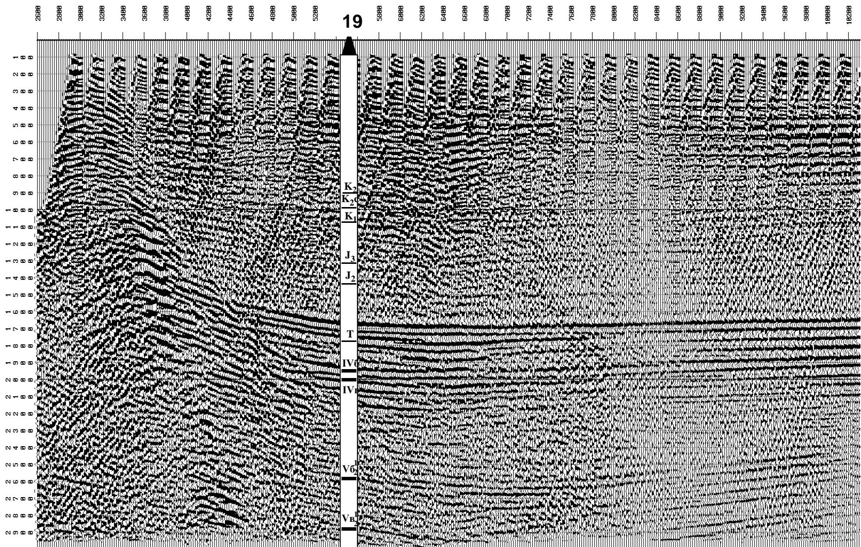
**Synthetic time cross-section** obtained for **the flank scheme** with receiver grouping on base  $l_G=120$  m and interval between centers of a group  $\Delta X_{RP}=40$  m (magnified scale).
