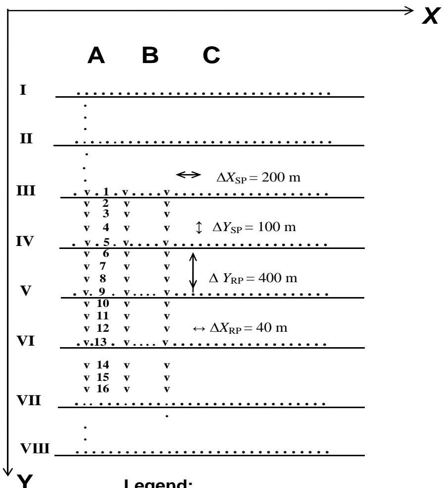
**Variant 2.** Survey geometry of “cross” type with 8 lines in the swath
