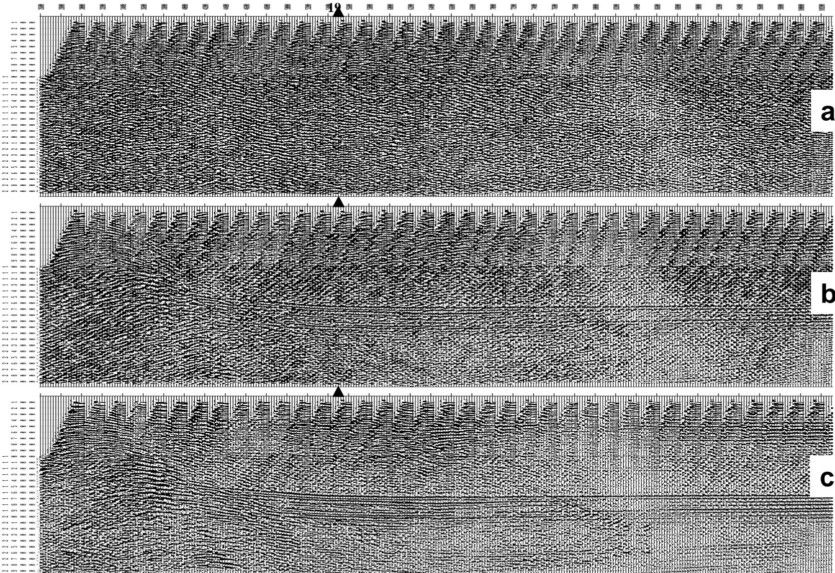
Comparison of synthetic time cross-sections obtained for **the flank scheme** with step between **centers of groups**  $\Delta X_{RP}=50$  m: a – without receivers grouping; b – grouping of receivers on base  $I_G=50$  m; c - grouping of receivers on base  $I_G=150$  m.
