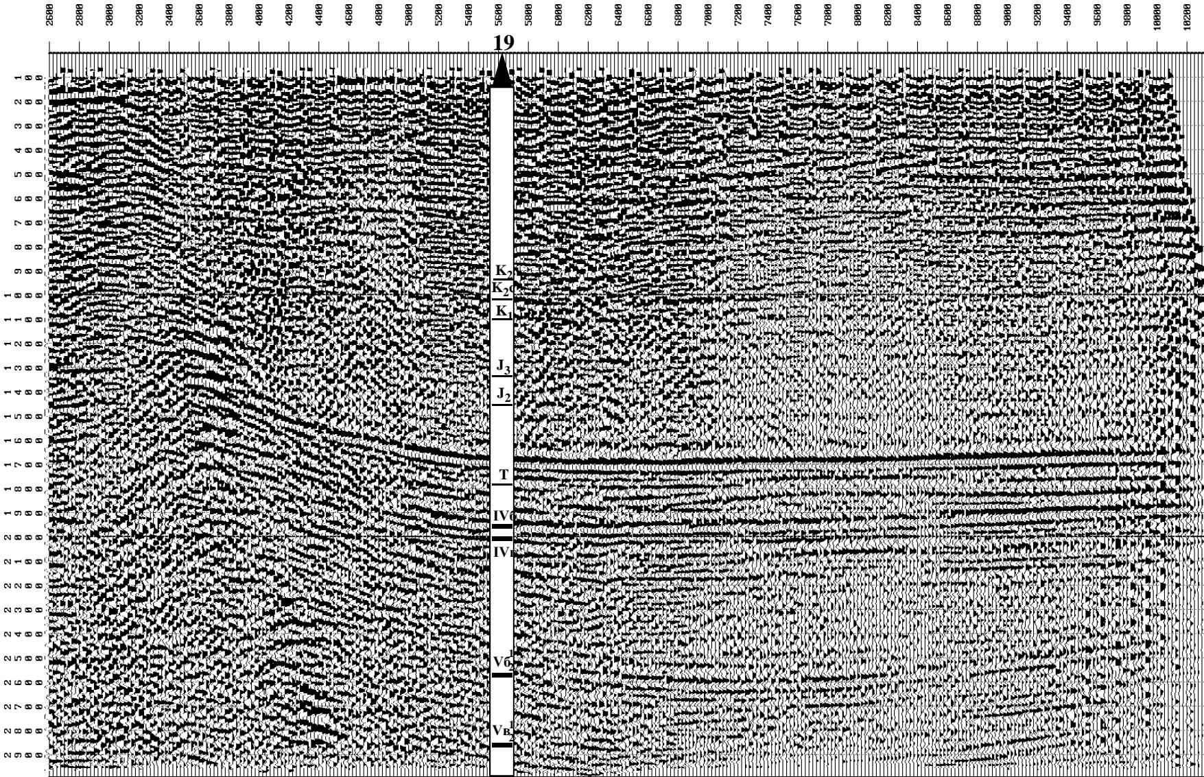
**Synthetic time cross-section** obtained after subtraction of multiples by Berchhaut algorithm. **The central scheme** with receiver grouping on base  $l_G=150$  m and interval between centers of a group  $\Delta X_{RP}=50$  m is used (magnified scale).
