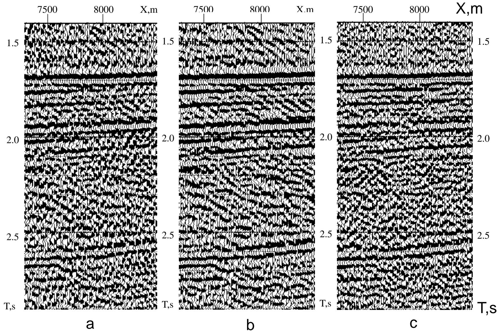
**Testing of program of surface waves-hindrances suppression:** **a** – time cross-section without surface waves-hindrances suppression; **b** – time cross-section with suppression of surface waves-hindrances basing on the F-K filtration; **c** – time cross-section with suppression of surface waves-hindrances basing on a singular decomposition.
