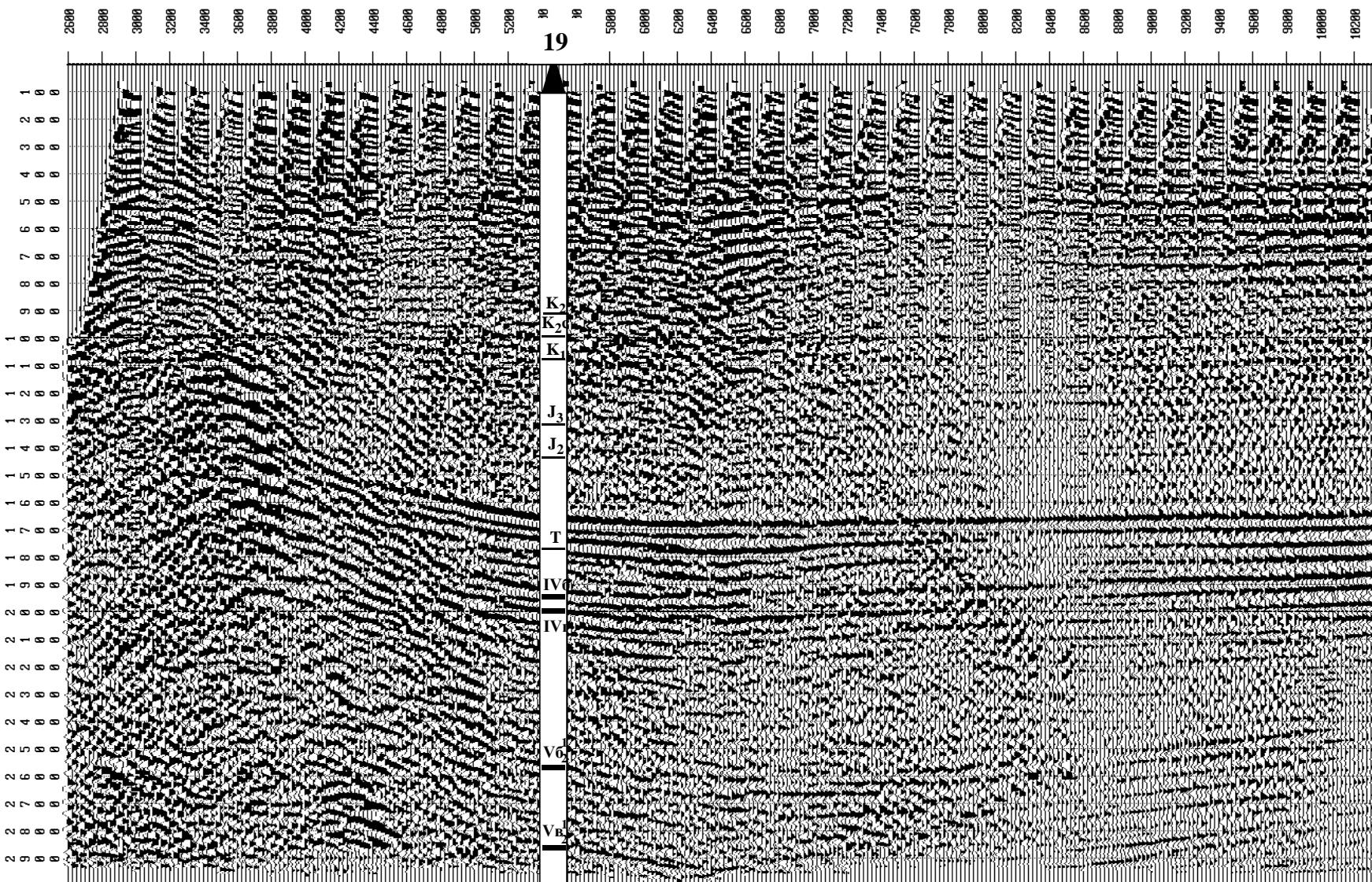
**Synthetic time cross-section** obtained for **the flank scheme** with receiver grouping on base  $I_G=150$  m and interval between centers of a group  $\Delta X_{RP}=50$  m (magnified scale).
