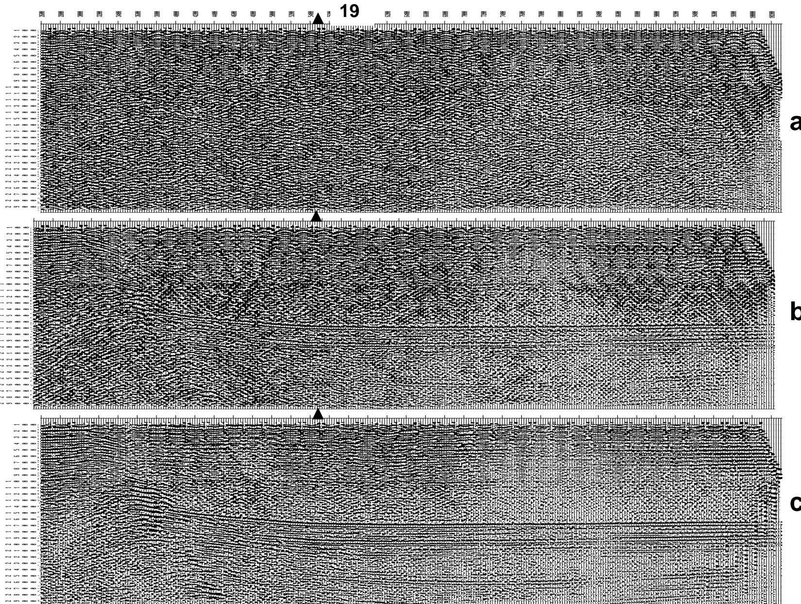
**Comparison of synthetic time cross-sections** obtained for **the central scheme** with step between **centers of groups**  $\Delta X_{RP}=40$  m: a – without receivers grouping; b – grouping of receivers on base  $I_G=50$  m; c - grouping of receivers on base  $I_G=150$  m.
