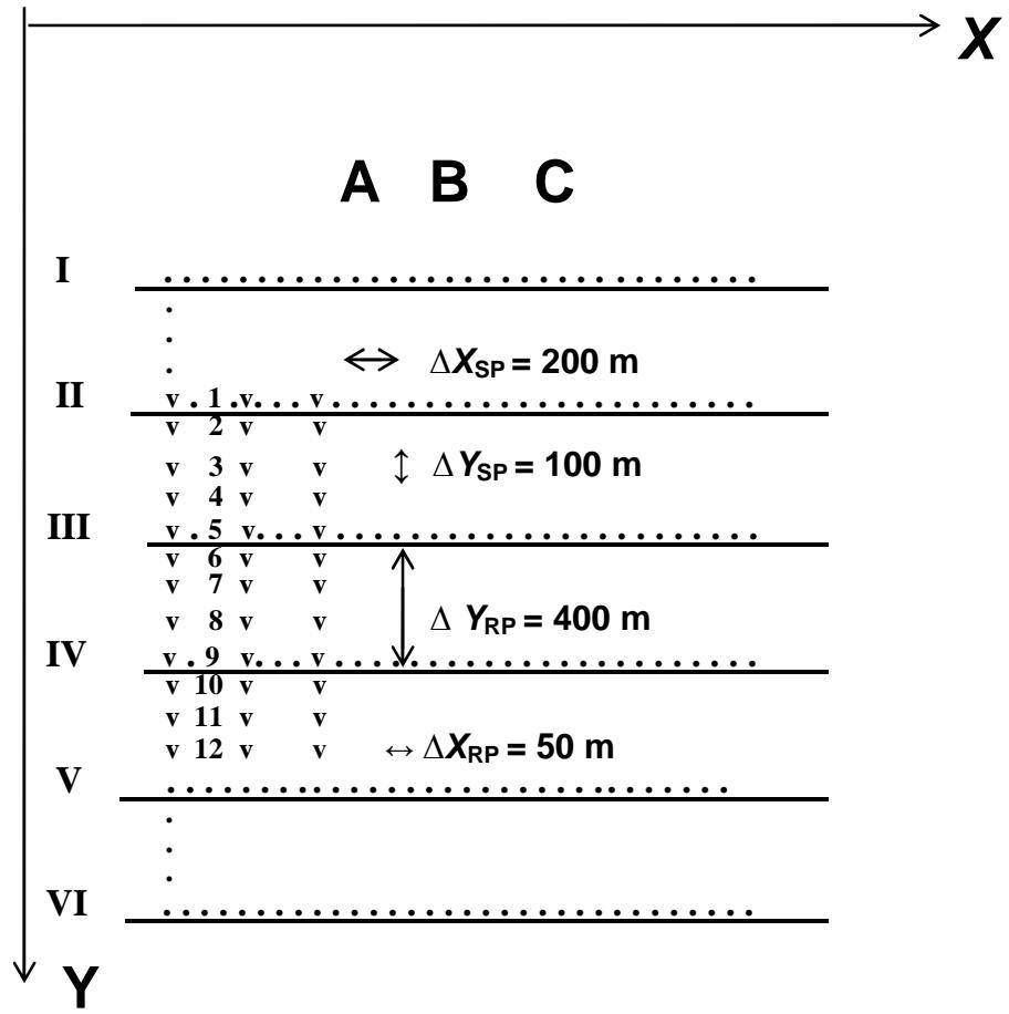
**Variant 1.** Survey geometry of “cross” type with 6 lines in the swath
