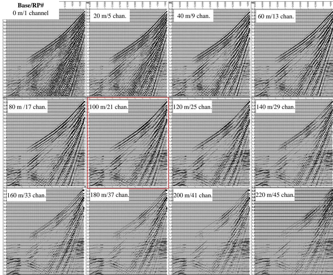
**Samplings** of receiver grouping base for **the flank** scheme (Elastic medium model)
